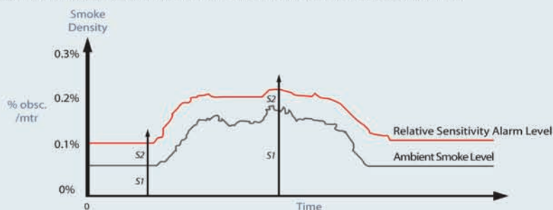
Fig. 1 Relative Sensitivity - shows how the value S2 is "Relative" to the variable ambient value S1
